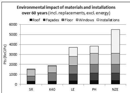
FIGURE 7 – ENVIRONMENTAL IMPACT OF MATERIALS AND INSTALLATIONS OVER LIFE CYCLE FOR DIFFERENT RENOVATION SCENARIOS
