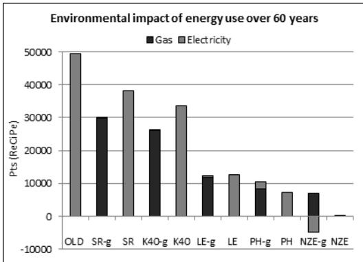
**FIGURE 9** – ENVIRONMENTAL IMPACT OF ENERGY USE OVER LIFE CYCLE FOR RENOVATION SCENARIOS WITH NATURAL GAS COMPARED TO ELECTRICITY AS ENERGY CARRIER FOR HEATING
